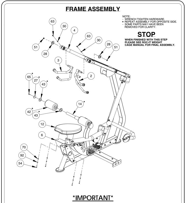
NOW THAT THE RS-1201-A IS COMPLETELY ASSEMBLED TAKE TIME TO ASSURE THAT YOUR UNIT IS ASSEMBLED SQUARE AND PERPENDICULAR. IF NOT, IT WILL BE NECESSARY TO LOOSEN SOME FRAME HARDWARE TO RE-ALIGN THE FRAME AND RETIGHTEN BOLTS.
