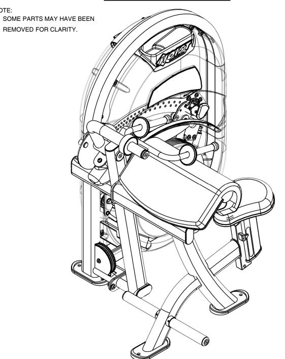
\*\*WRENCH TIGHTEN ALL PREVIOUSLY HAND TIGHTENED HARDWARE.\*\* NOW THAT THE CL-3103 FRAME IS COMPLETELY ASSEMBLED, TAKE TIME TO ASSURE THAT YOUR UNIT IS ASSEMBLED SQUARE AND PERPINDICULAR. IF NOT, IT MAY BE NECESSARY TO LOOSEN SOME FRAME HARDWARE TO RE-ALIGN AND THEN RE-TIGHTEN THE BOLTS
